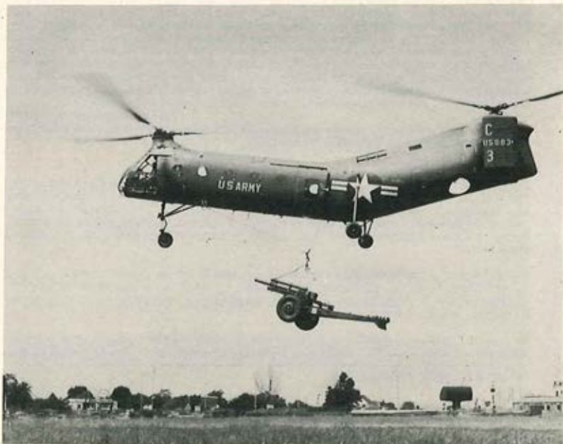
PIASECKI ARMY H-21C "WORK HORSE" LIFTING A TWO-TON 105-MM HOWITZER (Story Above)
