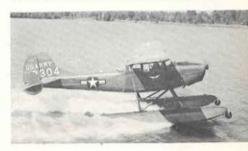
to the apparatus. The amphibious floats are designed to provide the capability of landing on water or land at the pilot's option.
