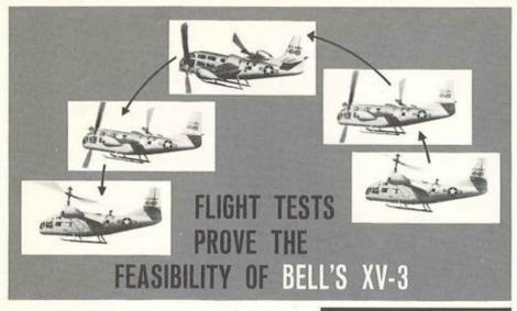
Over 100 hours of flying time by eleven pilots (2 AFFTC, 5 NASA, 4 Bell), have recently substantiated Bell's fixed-wing/prop-rotor concept. They showed again the advantages of the XV-3's optimum combination of helicopter and airplane flight characteristics.
