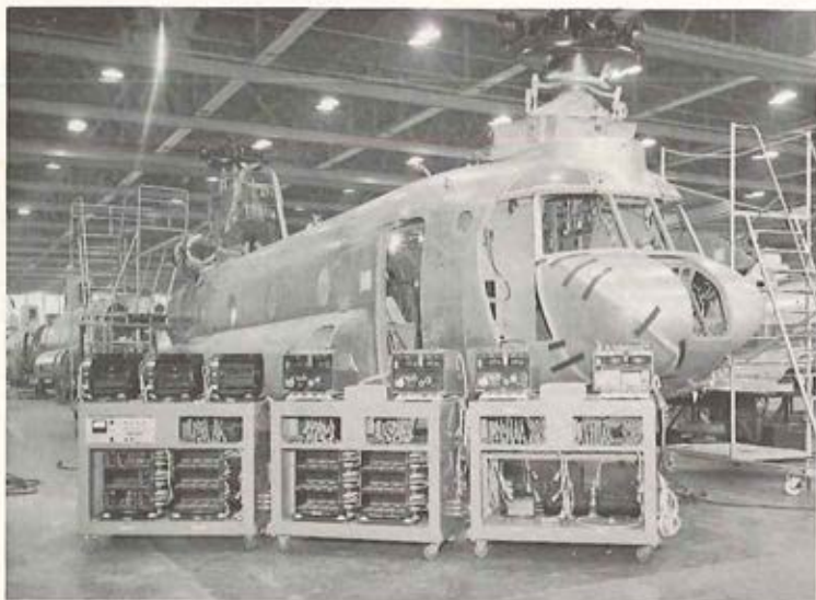
Slide-In Flight Test Instrumentation Racks
