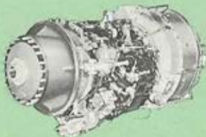
Lycoming T-53-L-1 gas turbine engine provides military rated 860 shaft horsepower.
