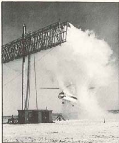
LEFT: An electrical rotor blade de-icing system undergoes rigorous testing on the blades of a Boeing Vertol 107 at Canada's National Research Council facility near Ottawa, Canada. A spray-rig (left) produces a vapor cloud which condenses on the rotor blades while sub-freezing Canadian weather quickly reduces this moisture to ice. Heated strips running along the blades' leading edges cause the ice to loosen and the whirling motion of the rotor blades sheds the thawing ice. BELOW: President Kennedy's car leads an entourage of distinguished military and civilian leaders before an array of the 1st Armored Division aircraft. The review at Ft. Stewart, Ga., took place during the division's recent STRAC (Strategic Army Corps) mobility exercise. (USA photo)
