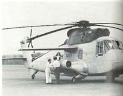
High-speed compound S-61F. A valuable step toward AAFSS, it embodies the Sikorsky concept of a FLEX-ROTOR.
