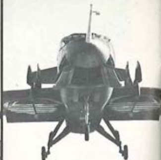
GE-Ryan XV-5A lift fan system J85 engine
