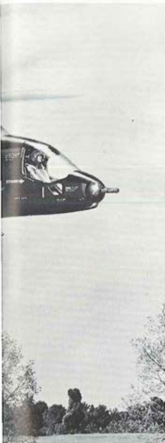
High-speed compound S-61F, with same gross weight as the AAFSS, is currently in test flight. It embodies the FLEX-ROTOR and unloaded rotor concepts, both pioneered by Sikorsky.
