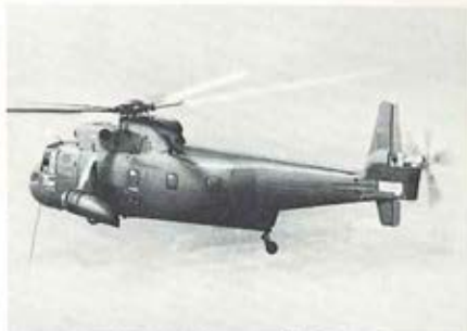
Sikorsky ROTOPROP in highly successful flight test. It serves as a conventional tail rotor at hover and low speeds, then swivels 90° aft, as shown, to provide forward thrust.
