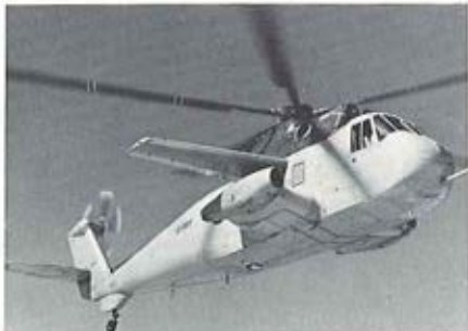
High-speed compound S-61F, with same gross weight as the AAFSS, is currently in test flight. It embodies the FLEX-ROTOR and unloaded rotor concepts, both pioneered by Sikorsky.
