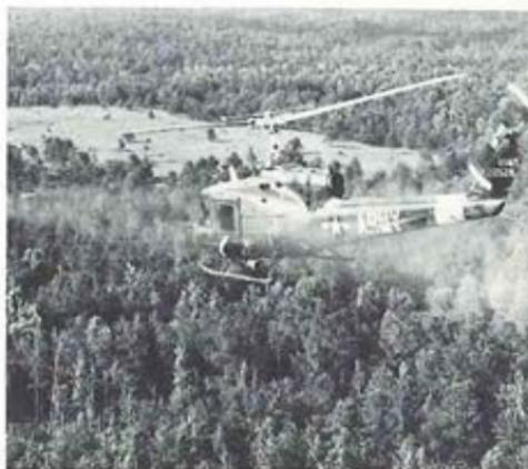
Daylight gunnery begins with the four 7.62-mm machine guns, two on each side of the UH-1.
