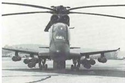
STRATFORD, CONN. — Sikorsky Aircraft's S-67 Blackhawk demonstrates its firepower capability by carrying 152 2.75-inch anti-personnel rockets. They are designated FFAR for Folding Fin Aircraft Rockets. The turret beneath the fuselage can carry either 20mm or 30mm cannon. The Blackhawk, the world's fastest helicopter, can also be equipped with other missiles and rockets to make it a highly lethal anti-tank weapons system. Among this armament is the TOW missile system.
