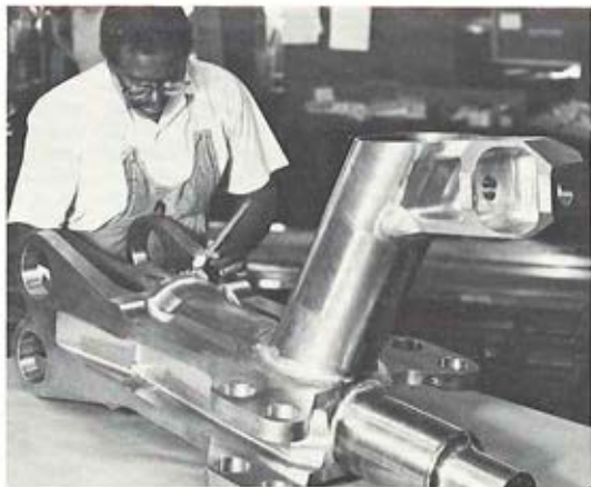
600 operations later the rough forging has been transformed into this complicated precision machined Pitch Housing Assembly weighing 236 pounds.
