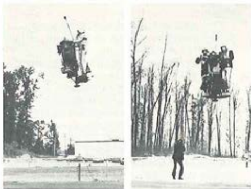
WALLED LAKE, MI.—Initial flight tests of the one- and two-man WASP (Williams Aerial Systems Platform) are underway. Fanjet-powered, the Williams Research Corporation's flying platform is designed to fly one or two men for 30 minutes at 60 mph speeds. Flown here on a safety tether line - used during early trial tests - by test pilot Robert Courter [left photo] and with passenger Jack Benson [r.], the WASP was built under a Navy contract as a candidate for the Marine Corps' Small Tactical Aerial Mobility Platform [STAMP].
