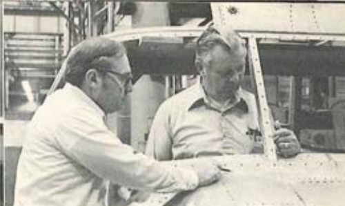
ARPRO-BV Inspectors Mr. Kirchhoff and Mr. Carey accomplishing inspection of modification rework on cockpit section of 001 aircraft.
