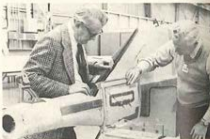
ARPRO-BV INSPECTORS, MR. WELSH AND MR. TASKER, ACCOMPLISHING AN INSPECTION ON THE CH-47D COMPOSITE BLADE FOR CONDUCTOR STRAP BONDING.
