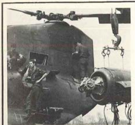
POWER SERVICE —PVT Donald Skulich (sitting) and SP4 Roger Anderson wait for PVT Michael Bailey to put the finishing touches on a Chinook's port engine so they can remount it on the bird. The men of Co C, 158th Avn Bn serviced the CH-47 from stem to stern during a phase maintenance operation. The 101st Abn unit did the "switch" during an April 3-14 field exercise near Russellville, Kentucky.
