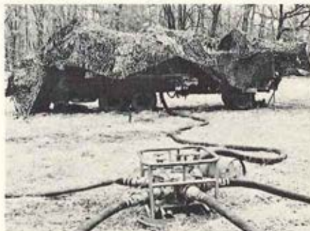
A truck-borne Rapid Refueling Point (RRP) package is shown in a field site in the "ready-to-pump" position. ■
