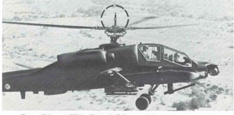
From -50 kts. to +200 kts. Three-axis. Fully compatible with other mast-mounted sensors. Provided with angle-of-attack sensing and anti-icing.
