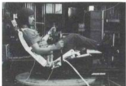
A soldier experiences simulated vehicle vibration in evaluation of occupational muscle stress during USAARL's vibration research program. The bite-bar (in the mouth) measures linear and rotational acceleration.
