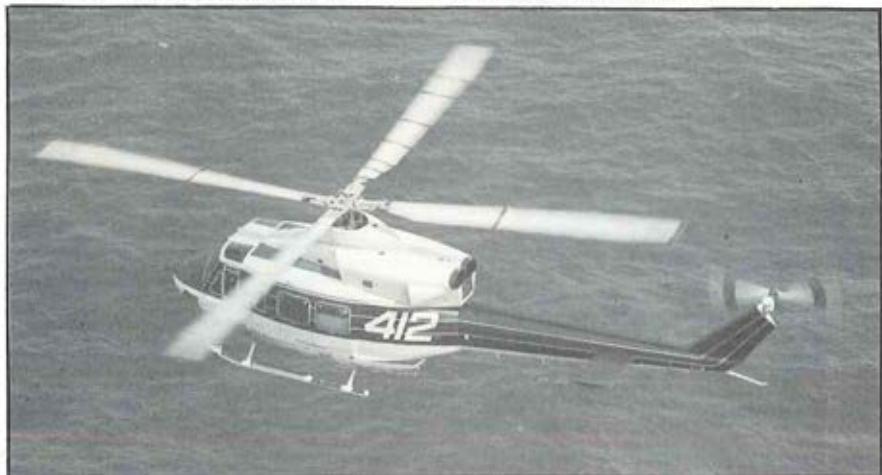
FIGURE 2—THE AHIP MAIN ROTOR WILL BE A SCALED DOWN VERSION OF THE CIVIL CERTIFIED MODEL 412 ROTOR SHOWN ABOVE.
