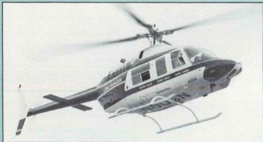
FIGURE 1—THE SOFT-IN-PLANE, FLEX-BEAM 4-BLADED BELL-DESIGNED ROTOR WAS DEVELOPED ON THE BELL MODEL 206-LM.
