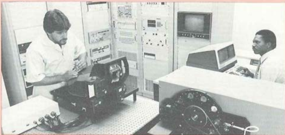
ABOVE: PNVS COMPUTERIZED ALIGNMENT AND TEST STATION.
