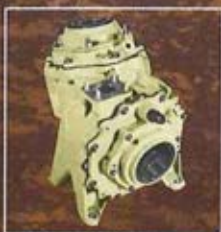
Intermediate Gearbox. Grease lubricated. Ballistically tolerant.
