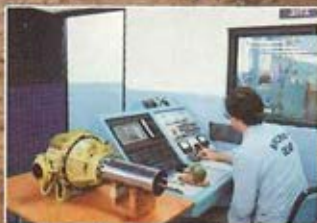
Tail Rotor Gearbox. Grease lubricated.
