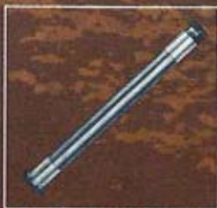
Main Rotor Drive Shaft. Nitalloy N and maraging steel. Inertia welded.
