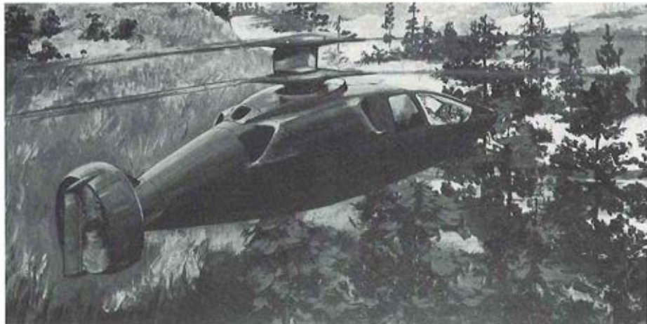
ABOVE: An early conceptual rendering of a high-speed Sikorsky LHX featured a single-pilot, twin-turbines, pusher propeller, and an Advancing Blade Concept (ABC) co-axial rigid rotor system.
