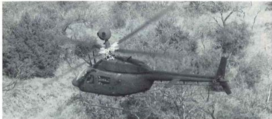
ABOVE: An OH-58D AHIP scout helicopter prototype in nap-of-the-earth flight. OPPOSITE PAGE: An OH-58D masking behind trees exposes only the 26" diameter of it's Mast Mounted Sight.
