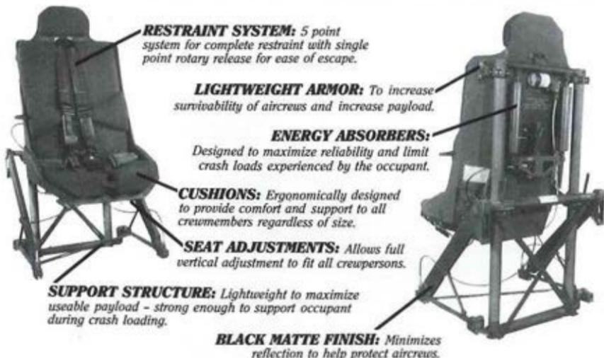
Increased survivability is the name of the game. Energy-attenuating seating systems by Simula can provide an extra measure of protection to crewmembers in a crash situation. Each component of our energy-absorbing crewseats is thoroughly engineered to work together as a system - from the energy-absorbing load attenuators to the ergonomically designed bucket.
