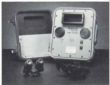
With the new ANV-20/20 from Hoffman Engineering, you can find infinity in the field, on the flight line, or in the back of a transport. This compact, battery operated system allows accurate adjustment of infinity focus, assessment of high and low light resolution, and a visual check for NVD dynamic range.....All in one portable package!
