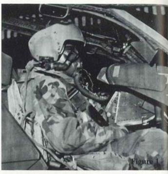
ponents is 57 pounds. Figure 1 (on the right) shows the same aviator in the front seat of an AH-64A Apache. Note how close he is to the Optical Relay Tube (ORT) and the digital keypad he is expected to use. We have failed in the integration or systems engineering of the human as a system.
