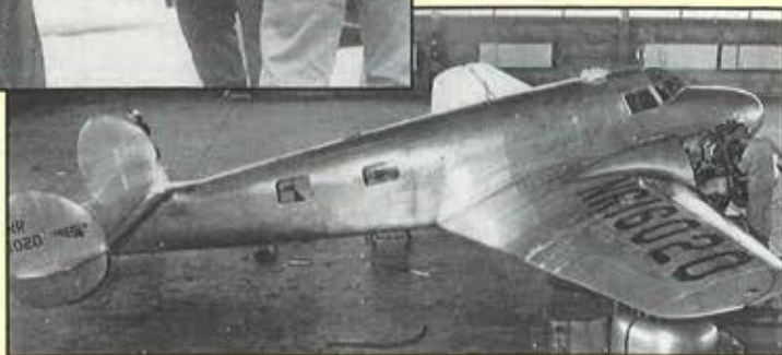
Bottom: Earhart's Lockheed Vega, fully assembled by Army aircraft mechanics in a Wheeler Field hangar. The plane was shipped to Hawaii in major assemblies.
