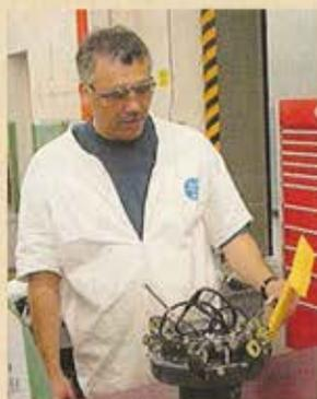
Rudy Lopez, an aircraft mechanical parts repairer/mechanic, reviews final paperwork after the swashplate's assembly and before the item is ready for final painting.
