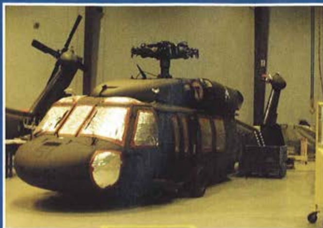
The third production UH-60A Black Hawk as received at Troy; its main landing gear struts are deflated for trailer transport.
