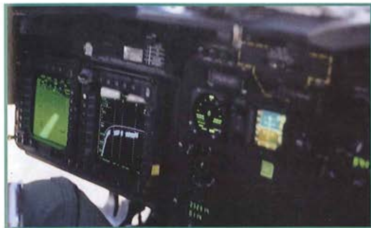
Very "clean" cockpit with all aircraft system warnings, cautions and advisories monitored and displayed through the Integrated Avionics Program on the Multi-Function Displays.
