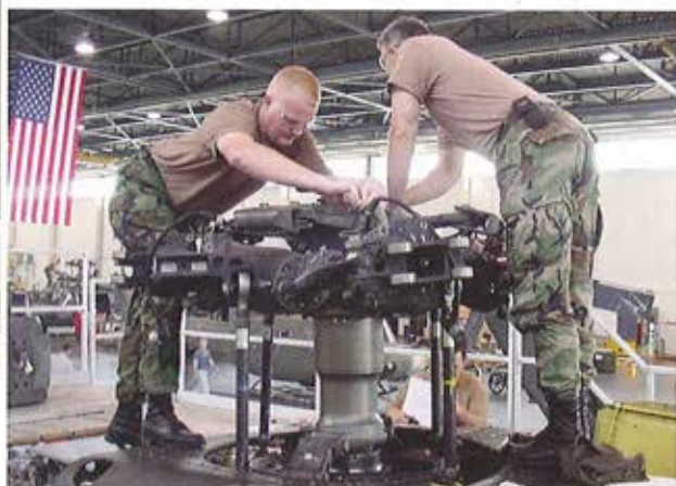
Gulfport, Miss., students in the USAALS UH-60 Road Show program install a main rotor de-ice distributor on a Black Hawk.
