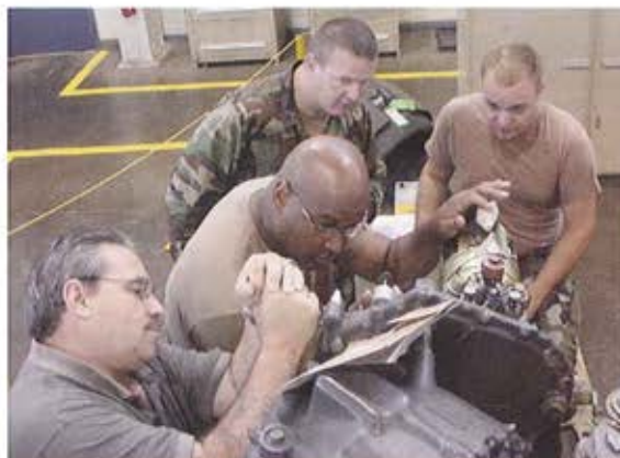
Gulfport students remove a main generator spline adaptor under supervision of Road Show instructor Nolan Billiot.
