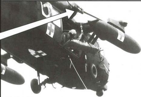
BREEZE-EASTERN's high performance, external rescue hoist system has met the stringent qualifications of the UH-60Q MEDEVAC program. The HS-29900 delivers the highest operating performance of any rescue hoist on the market today, with faster cable speed (350 fpm), longer cable (295 feet) and unlimited duty cycle.
