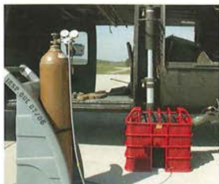
The new protection cage and safety device for servicing aircraft tires.
