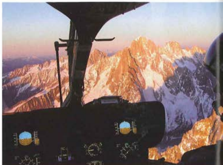
The advanced, night vision-compatible glass cockpit with the vehicle and engine management displays (VEMD) enhances situational awareness while reducing pilot workload. EADS PHOTO COURTESY
