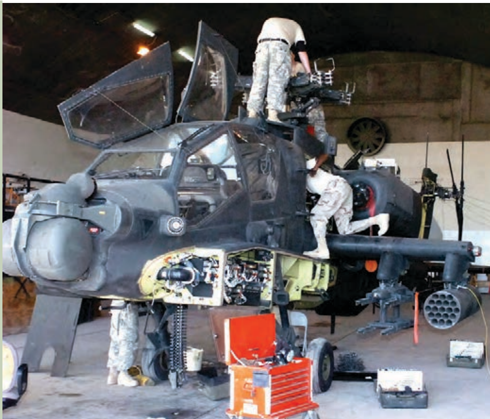
The aviation maintenance technician is the unit commander's maintenance manager and planner, ensuring aircraft readiness to meet operational tempo demands. Here Soldiers with Co. B, 935th Avn. Spt. Bn., Missouri ARNG, perform a 250-hour phase inspection on an AH-64 Apache Dec. 14 in Iraq. ARMY PHOTO BY SSG LORIN T. SMITH
