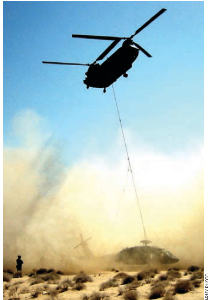
Soldiers from the downed aircraft recovery team of Co. B, 449th Avn. Spt. Bn., recover a UH-60 Black Hawk Nov. 9 belonging to the 36th Cbt. Avn. Bde. after the helicopter made a precautionary landing in Southern Iraq because of low fluid pressure. The 36th CAB is one of the units receiving the ULLS-AE system software and hardware in FY06.
