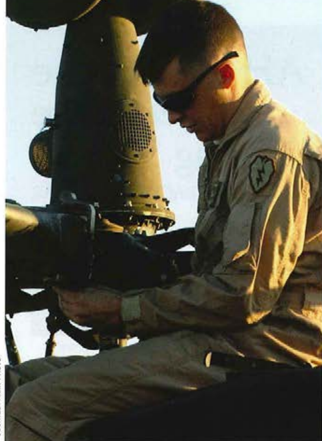
Crew chief SPC Kevin McMahon with Troop C, 2nd Sqdn., 6th Cav. Regt., replaces expanding bolts on an OH-58D Kiowa helicopter Jan. 18 near Kirkuk, Iraq. AMCOM has made major strides with working condition based maintenance with the goal of reducing the workload of Soldiers and improving operational readiness rates across the aviation fleet.
