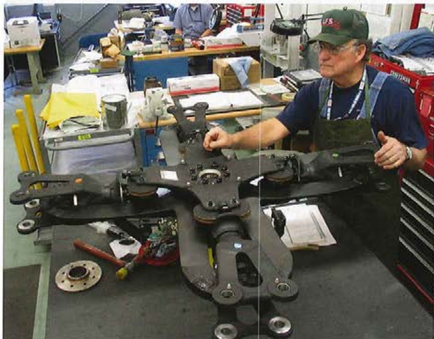
The Aviation Center Logistics Command at Fort Rucker plays a key role in the Army's National Maintenance Program by repairing parts, like this OH-58D Kiowa Warrior rotorhub, for the entire Army's supply program.
