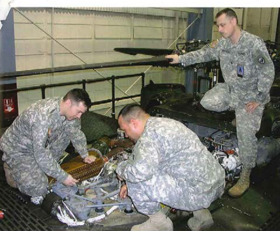
USAALS has revamped BNCOC making the training more in-depth and relevant to help develop a quality, trained NCO capable of effectively performing fundamental duties as a technical inspector. Here BNCOC students SGT Thomas Restuccio and SGT Aldo Dejesus (back to camera) conduct rigging pin installations and checks on the flight controls of a UH-60 as instructor SSG Bobby Curnutte observes.
