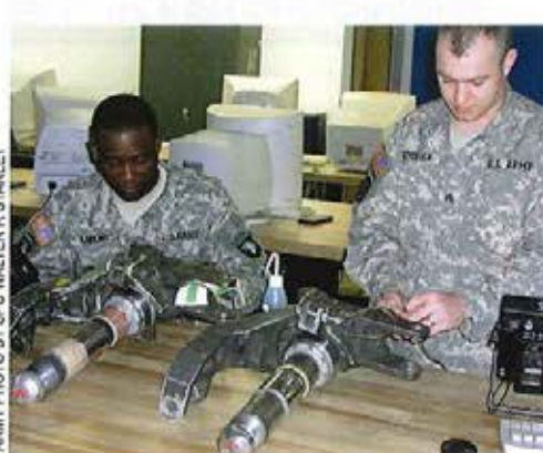
Basic NCO course students SGT Ashe Rawlins, left, and SGT Jonathan Kocurek perform an "eddy current test" as part of an inspection to check for cracks on spindle assemblies. Training on nondestructive testing (NDT) equipment and procedures has been consolidated and absorbed into the BNCOC for the 15D aircraft power train repairer skills training at Fort Eustis.
