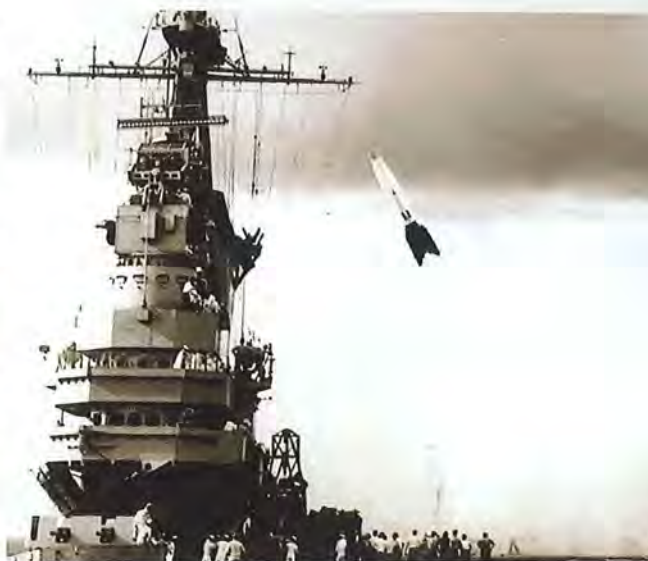
ABOVE: On Sept. 6, 1947, a V-2 was launched off the after flight deck of the USS Midway as part of "Operation Sandy," a joint Army-Navy test. It exploded at an altitude of 5,000 feet before accidentally exploding in flight. As a result, the Navy decided to pursue solid fuel rockets instead of liquid fuel rockets. LEFT: German Maj. Gen. Walter Dornberger (1), commander of the German V-2 rocket development program; with Lt. Col. Herbert Axter (2); Professor Wernher von Braun (3); and Hans Lindenberg (4) on May 3, 1945, the day after they surrendered to U.S. troops in Austria. Von Braun broke his leg in a car accident several weeks prior to his surrender.
