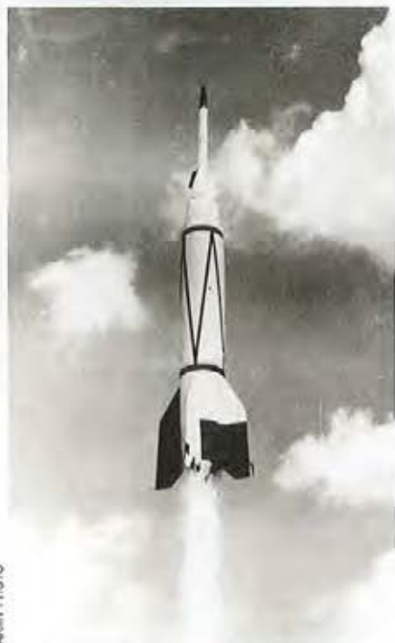
The "Bumper 5" during its Feb. 24, 1949 launch, it employed a V-2 missile as the first stage, and a pencil-like 700-lb rocket, known as a WAC (without altitude control) Corporal, as an upper stage.
