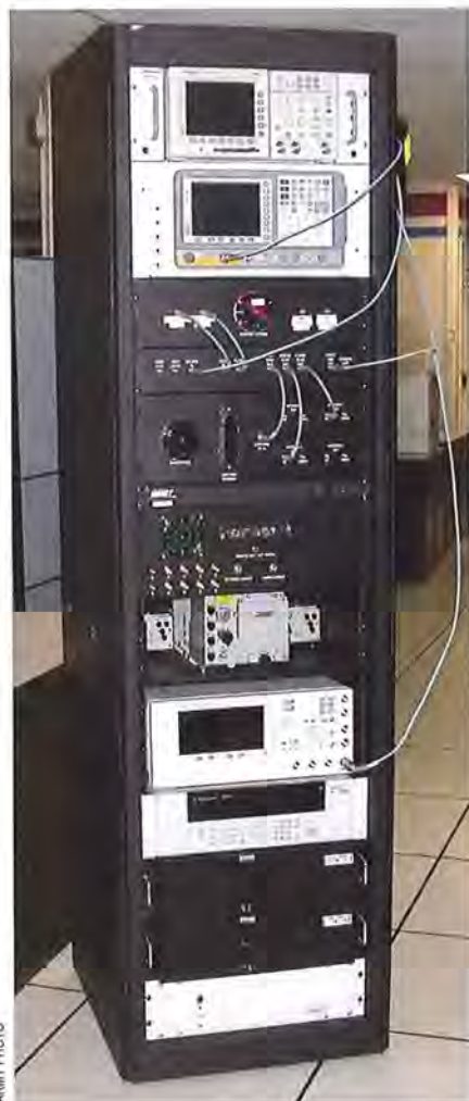
Figure 2: Simulation testing of mission data sets requires the use of high-fidelity radar signal simulators. Here is a test rack, controlled by the automation software, which selects the correct signal path based on test conditions for testing AN/APR-39 radar warning receivers.
