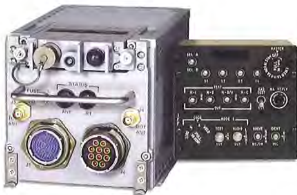
The Army's fixed wing fleet will be fielded with the AN/APX-119 transponder, also with Modes 1, 2, 3A, C, 4 and S.
