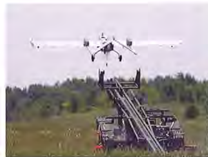
A Shadow 200 UAS launches on a mission with communication relay systems equipment installed aboard. The PIF conducted the CRS integration and testing.
