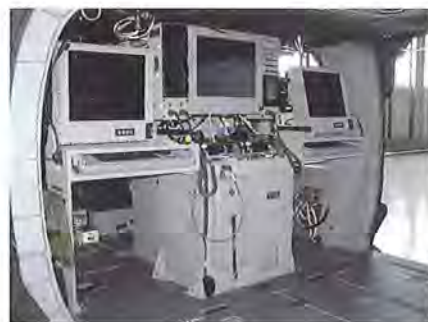
An Army airborne command and control system (A2C2S) workstation is installed inside the forward cargo area of a UH-60 Black Hawk helicopter.
