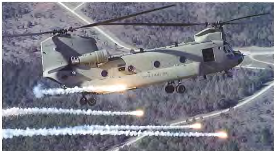
The program director for aircraft survivability equipment is providing the aviation warfighter with the latest upgrades and enhancements to the common missile warning system and the improved countermeasure dispenser. Here, a system test is conducted on the new CH-47F model Chinook to verify operability.
