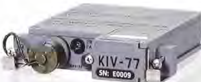
The KIV-77 is the Mode 4 and 5 appliqué for the AN/APX-119 used with fixed wing aircraft.
