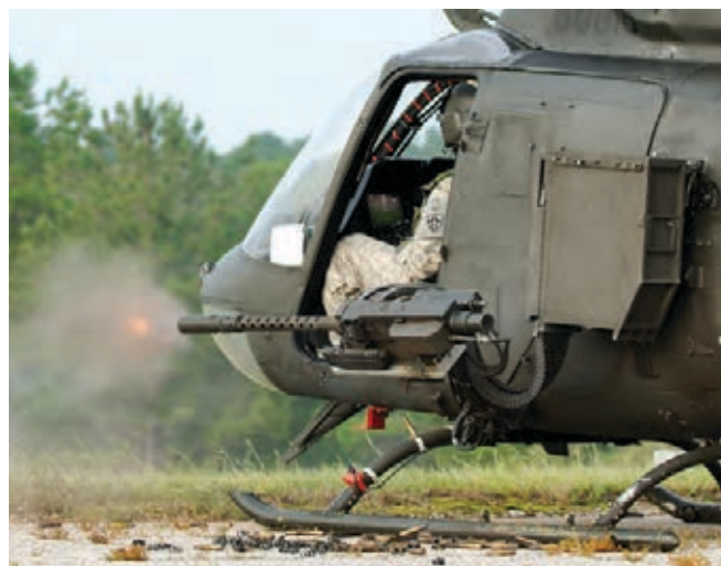
The Army Aviation Technical Test Center in conjunction with the ASH Project Office helped to test the M3P .50-caliber machinegun for the force.
