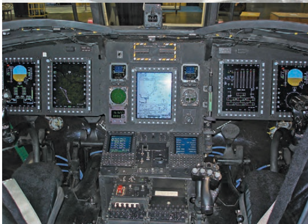
The new CH-47F model uses the common avionics architecture system (CAAS) "glass" cockpit with multifunctional displays.
