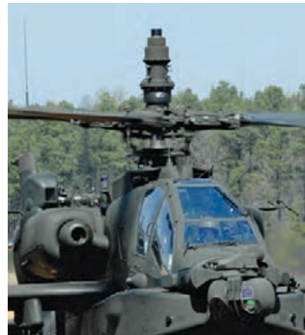
PM Apache helped with the development of the VUIT-2 system (note antenna array mounted on the rotor masthead) which provides pilots with real time UAS video feeds into the cockpits of the aircraft. Here, LTC Charles Walls with the Aviation Applied Technology Directorate tests the interoperability of the system from the front seat of the Longbow at Fort Pickett, Va.
