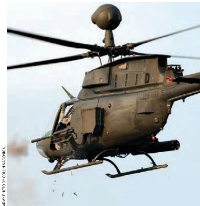
An OH-58D Kiowa Warrior fires the M3P machinegun during developmental flight testing at Matteson Aerial Gunnery Range, Fort Rucker, Ala.
