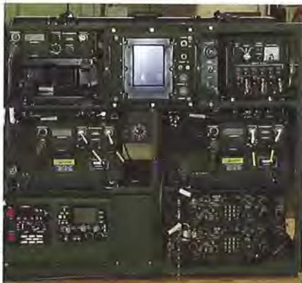
Tactical Terminal Control System (TTCS) new modification work order (MWO) configuration.
