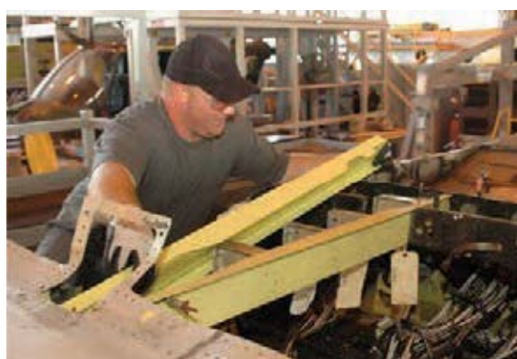
One of CCAD's aircraft production artisans installs the locally manufactured main cabin roof beam into the OH-58D Kiowa Warrior Pilot Program helicopter.
