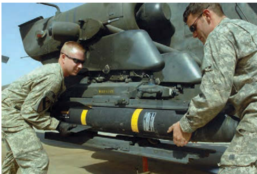
SPC Sean McConnell (left), of Columbus, Ohio, and SPC Scott Shaver, of Austin, Texas, load a Hellfire missile onto the mounting bracket on an AH-64D Apache helicopter in Camp Taji, Iraq, Oct. 1. Both Soldiers are armament electrical avionics repairers assigned to Company D, 1st Battalion, 227th Aviation Regiment.
