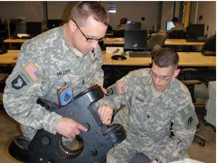
An MOS 15D powertrain instructor and student perform an eddy current inspection on a CH-47D rotor hub.
