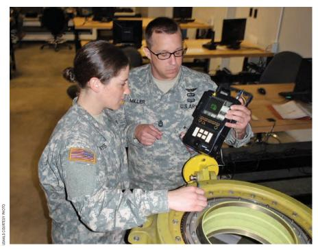
An MOS 15D powertrain instructor and student perform an eddy current inspection on a CH-47D swashplate.
