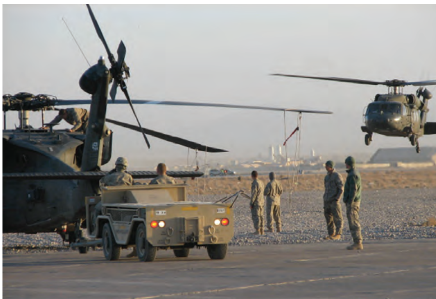
The Standard Aircraft Towing System in action.
