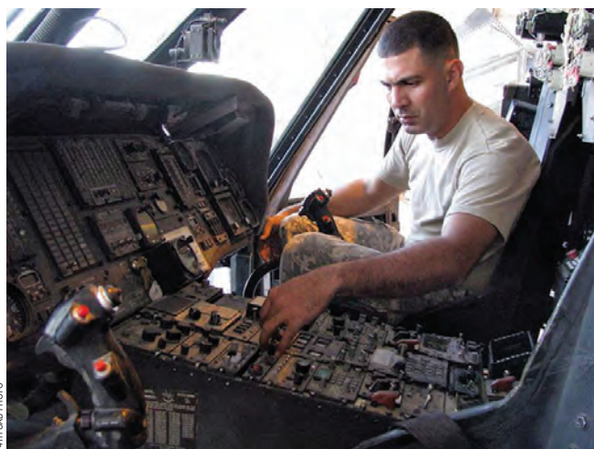
SPC Javier Garces troubleshoots the radios on a UH-60 Black Hawk. Garces is an avionics technician with Company B, 404th Aviation Support Battalion, 4th Combat Aviation Brigade, 4th Infantry Division.
