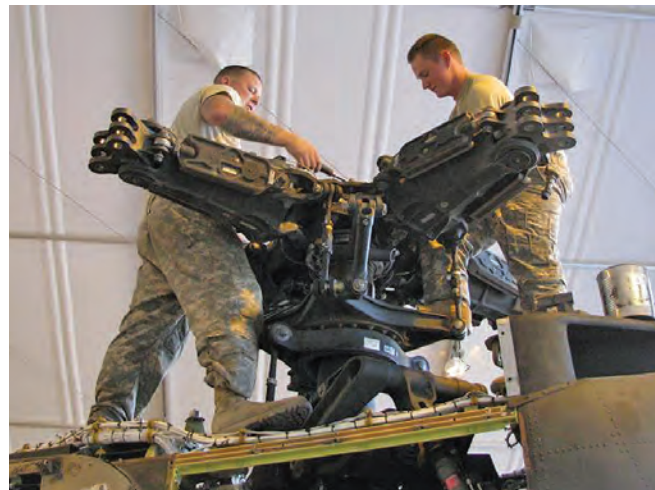
Camp Marmal, Afghanistan - Army Spc. Robert Huff, Mayfield, Ky., and Army Spc. Michael Pittsenbarger, Dayton, Texas, work on the rotor head of an AH-64D Apache helicopter. Both Soldiers are phase team leaders with Company B, 404th Aviation Support Battalion, 4th Combat Aviation Brigade, 4th Infantry Division and part of the Aviation Support Company. ASC performs phase maintenance on all aircraft in Task Force Mustang, 4th CAB's stable.
