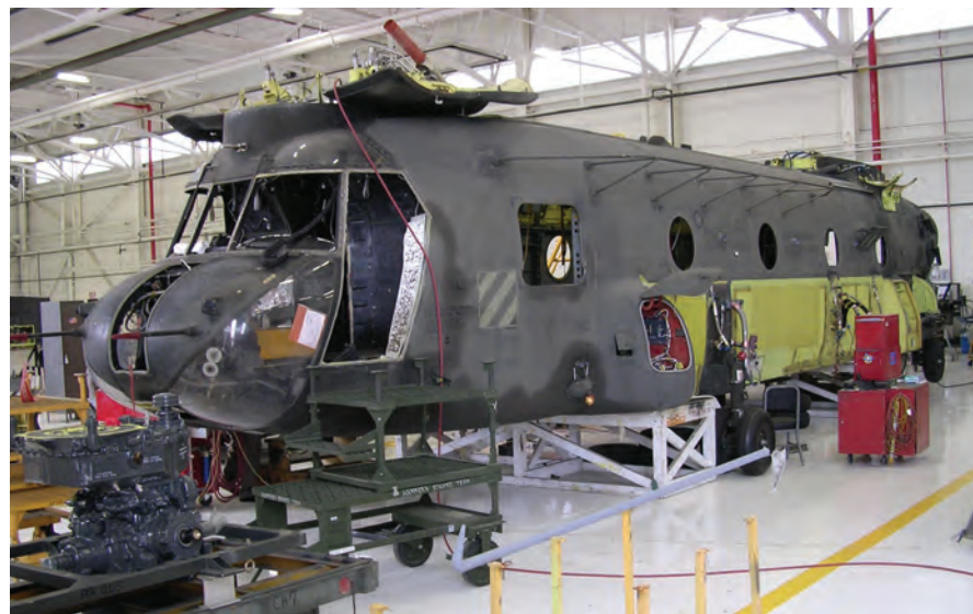
A CH-47 is disassembled and inspected during Reset; any structural faults will be corrected.
