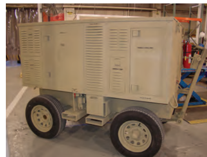
Aviation Ground Power Unit (AGPU)
