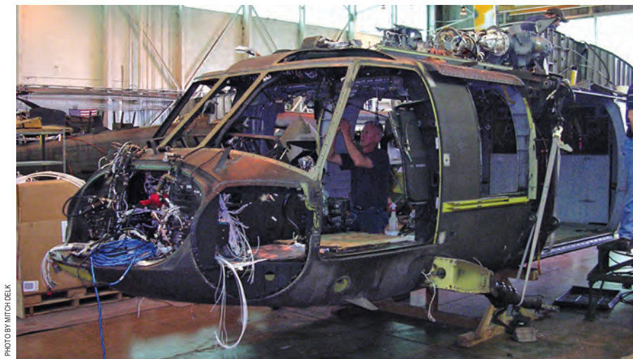
All aircraft are disassembled, thoroughly cleaned and inspected; a high percentage of aircraft require some type of depot level repair.
