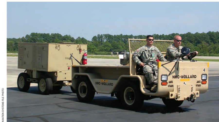
Standard Aircraft Towing System (SATS)
