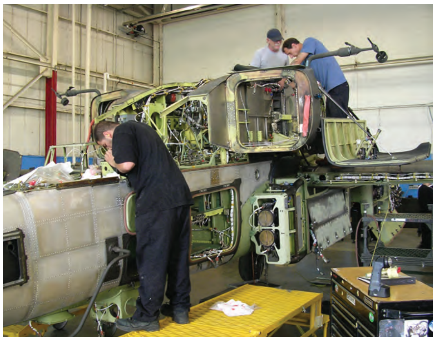
During Reset, dynamic components are repaired or replaced and any outstanding MWOs are applied as the aircraft is restored to fully mission capable status.
