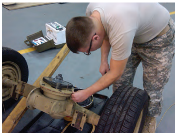
A soldier attending the 15H course inspects and prepares AGPU front axle for reassembly at Ft. Rucker, AL.
