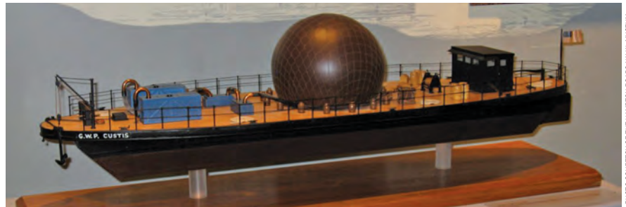
Model of the George Washington Parke Custis, flattop coal barge converted into a floating balloon carrier. Note gas-generating equipment mounted forward. The Custis was a forerunner of the modern aircraft carrier.
