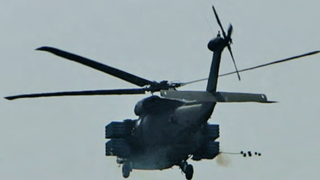
A UH-60 Blackhawk from the 2nd Bn., 2nd Cbt. Avn. Bde., disperses mines from its Air Volcano system during a capabilities exercise in Sept. 2010.
