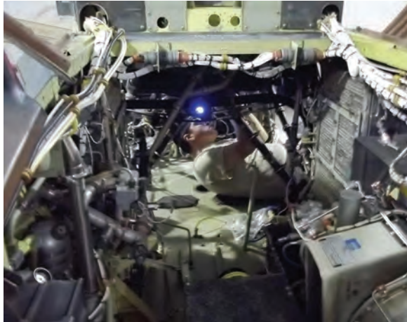
PFC Bryan Gomez, Co. D, TF 4-227th ARB performs phase maintenance in the main transmission deck area of an AH-64D Apache.
