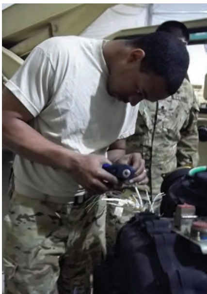
SPC Audrey Meekins of Co. D, TF 4-227th ARB wires an AH-64D Main Transmission prior to installation.
