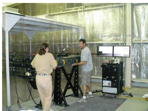
Dianne Simpson (JAMS engineer) and Jason Wilborn (contractor with Redstone Test Center) loading a HELLFIRE II missile on the test rail for evaluation on the Modernized HELLFIRE Test Set (MHUTS) for operation at the Forward Test and Repair Facility.
