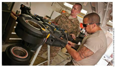
PV2 Norman F. Thompson, from Amherst, VA, and SPC Edwin Gonzales, of Humacao, Puerto Rico, both power train mechanics with the 122nd Aviation Support Battalion, Task Force Corsair, 82nd Cbt. Avn. Bde., perform maintenance on a CH-47 Chinook rotor head assembly at Forward Operating Base Shank, Afghanistan April 13.
