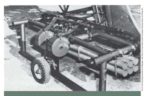
Dual mounting of machine guns and rockets on a U.S. Army H-13 Sioux helicopter.
