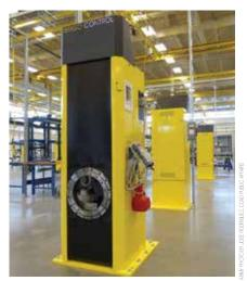
The DCRF's new transmission assembly stands can be used on most helicopter gearboxes. Employees can switch from working on a UH-60 transmission to an AH-64 transmission with only minor modifications. Its ergonomic design ensures the operator's overall comfort, health, and wellness.
