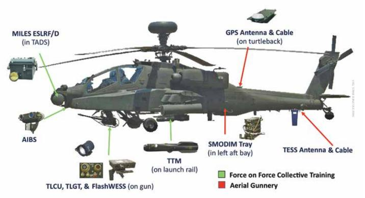
Figure 1. Longbow Tactical Engagement Simulation System (LB TESS)
