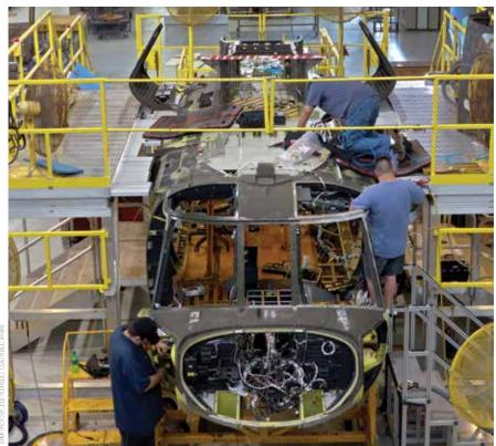
CCAD has several thriving programs to service H-60 helicopters in the joint services, to include the UH-60 recapitalization and crash damage repair programs. Black Hawks are disassembled to their bare components and prescribed a customized Statement of Work that will repair all wear and tear, and rebuild it with the most modern equipment, strengthening it for another decade of use.
