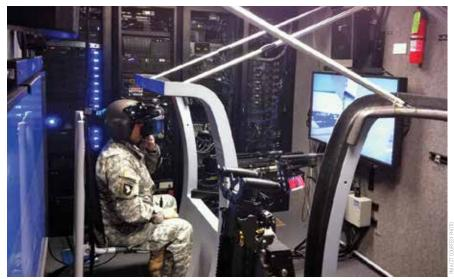
Non-rated crewmember training door gunnery in the Non-Rated Crewmember Manned Module (NCM3) utilizing helmet mounted displays.
